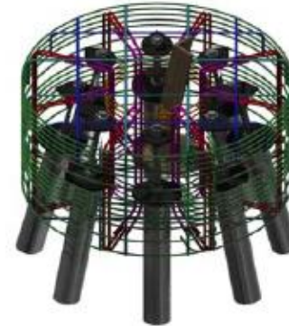
Micro Piles and Concrete Pile Cap
